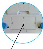
Battery compartment for the internal rechargeable battery with external access when needed
