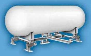
Horizontal Tank with End Discharge - The tank shown above is an example where the scale is mounted beneath the tank with an end discharge . Tank saddles are mounted directly to the scale girder chairs. If desired, tank saddles could be mounted to the scale weighbridge instead of directly to the scale.
