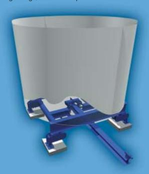
Vertical Tank with Flat Bottom - Scale is shown above with flat bottomed tank and side discharge. Main lever arms are connected under the tank area. Scales of this type are generally designed for use with light gauge flat bottomed tanks supported on timber or steel plate decks mounted on a steel weighbridge. However, if desired, scales may be designed to accomodate heavier gauge tanks without a steel weighbridge by mounting tank supports directly to scale girder chairs.
