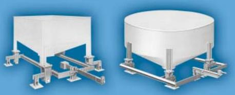
**Vertical Tanks with Cone Bottoms -** The scales shown above are examples of vertical tanks or hoppers with center discharges. Levers are so arranged with a center hookup and transverse lever outside of the scales which leave a center opening to permit discharge. Support legs of the hoppers can be mounted directly to the scale girder chairs or, if desired, a steel weighbridge could be used under the hoppers.
