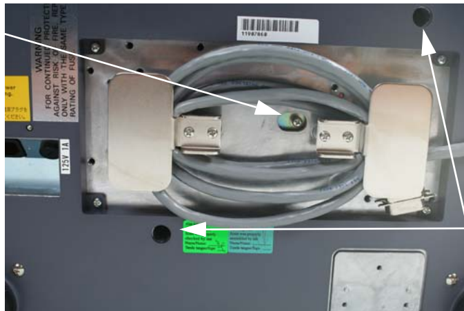
Figure 2-1. Location of Load Cell Setscrews for Single and Dual-Platform Scales (DIGI Scale Base shown)
