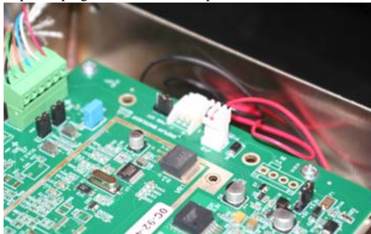
Figure 2-11. Connect Power Plug onto J12 on CPU Board
