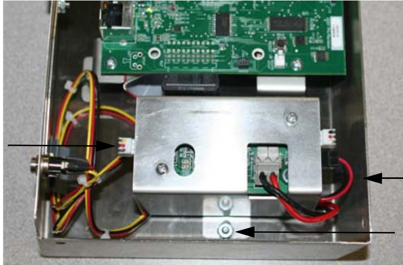
Figure 2-10. Secure Battery Pack into Enclosure
